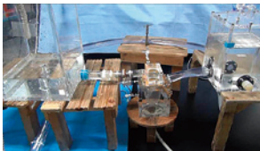
▲ Assessment of hydrodynamic features of a newly developed stentless mitral valve using a pulsation-type circulation system
