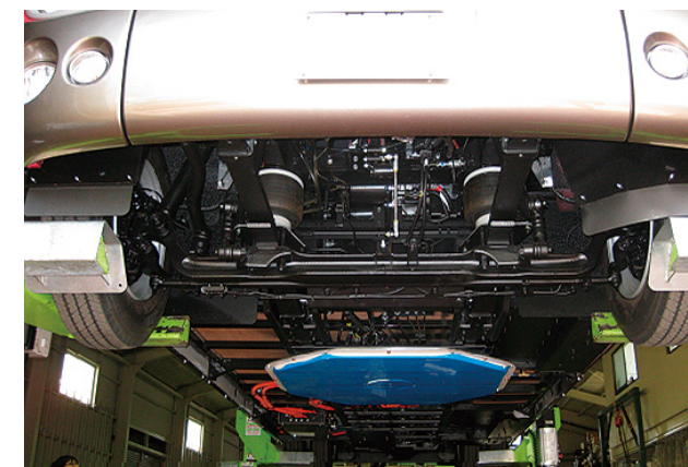
▲ Wireless charging device for electric vehicles
