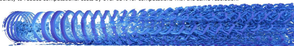
Figure 1: Efficient analysis of the wake of a wind turbine
