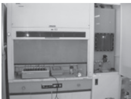
Figure 3-3-5. Fume hood equipped with a scrubber unit (scrubber equipment is shown on the right side)
