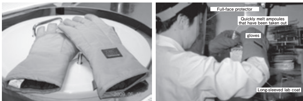
Figure 3-12-1. You should wear gloves, goggles and long-sleeved lab coat when handling liquid nitrogen
