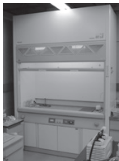
Figure 3-3-7. Fume hood equipped with activated charcoal (built-in activated charcoal cartridge at the top of the unit)
