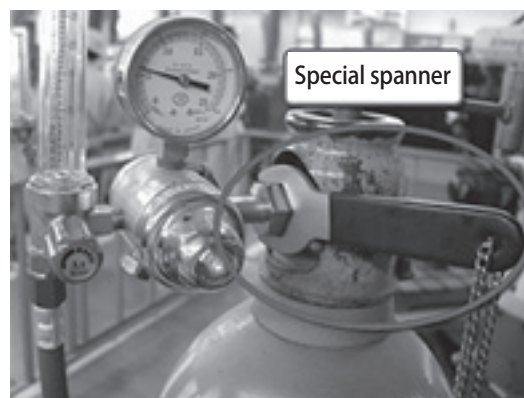
Figure 3-4-8. Handling pressure regulators
