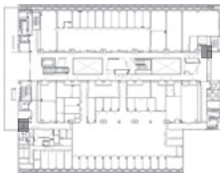
Figure 1-4-18. Locations of emergency showers on the 2 nd floor
