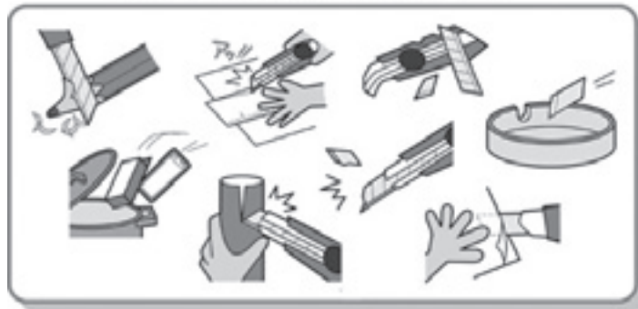
Figure 3-15-1. Examples of dangerous use (reference: NT Cutter website)
