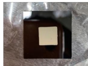
Ag aerogel film deposited on Si wafer in 2 minutes
