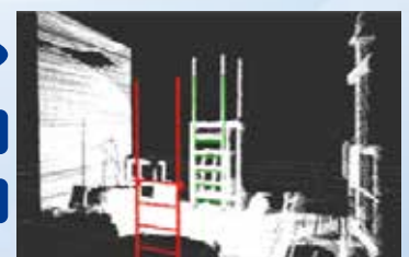
A model of a ladder (red) and the position and posture estimated ladder (green)
