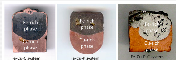
Fig.2 Copper enrichment process of low-grade copper scraps based on liquid phase separation
