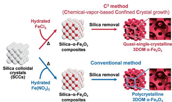
Fig. 1 塩化鉄の気相拡散と酸素との反応を経由した単結晶性 3DOM \alpha\text{-Fe}_2\text{O}_3 の合成. Adapted from Chemistry of Materials 2025, 37, 5005. Copyright 2025, American Chemical Society.
