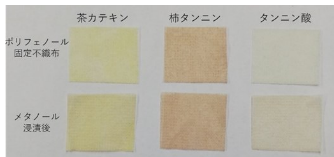
Fig. 7 Change of color after immersion of polyphenol-immobilized nonwoven fabrics in methanol
