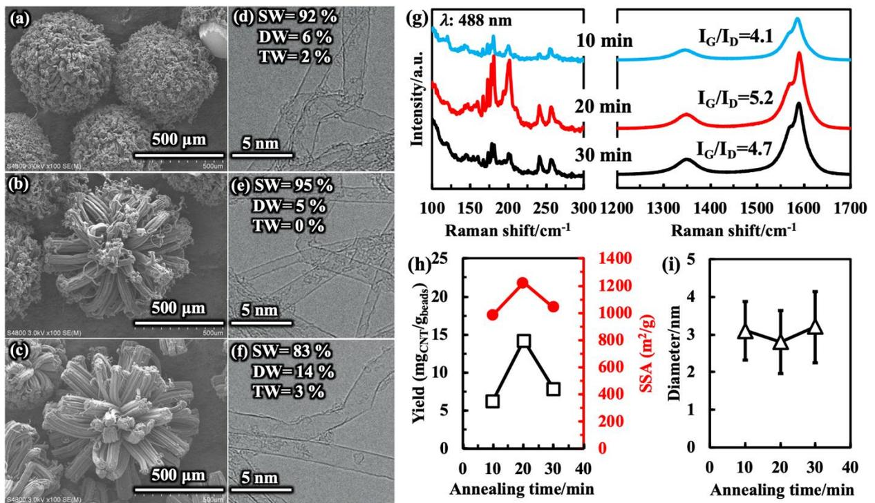
**Fig. 2** SWCNT arrays synthesized by FBCVD. (a-c) scanning electron microscope images, (b-f) transmission electron microscope images, (g) Raman spectroscopy, (h) yield and specific
