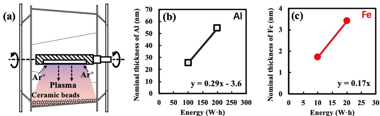
**Fig. 1** Schematic diagram of drum-sputtering facility and the measured deposition rate. (a) Schematic image of designed octagonal drum. Deposition rate of (b) Al layer sputtered at 120 W and (c) Fe layer sputtered at 20W performed by adding 100 g beads under Ar atmosphere for 60 min.
