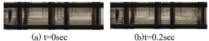
Fig.4 Flow Pattern ( \dot{m}=30\text{kg/h} , x=0.1 , Q=400\text{W} )
