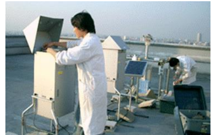
Small automatic solar-powered rainwater collector
